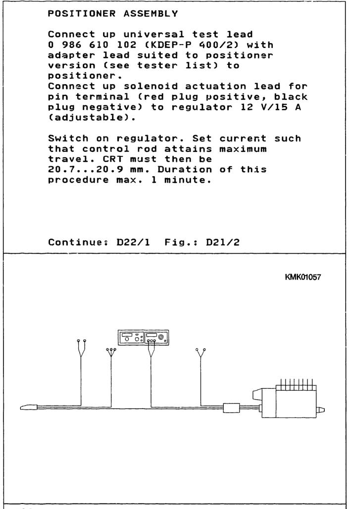
If this value is not correct, dimension "X" has been incorrectly calibrated (thrust pin in servo-magnet armature) and the procedure is thus to be repeated (measurement of dimension "X").
